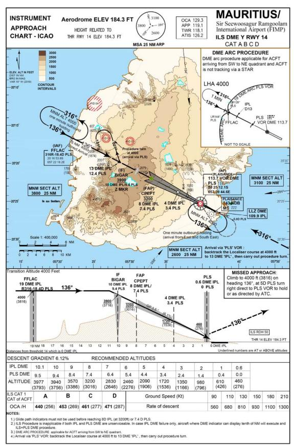
Changes: BIGAR is above 3900, CPEPT is @3200, obstacle elevations 2058 and 1674 added, underlined numbers are AT or ABOVE altitudes concern Profile, FFLAC is at 19nm from threshold in profile, Inclusion of Z MKR at BIGAR.
