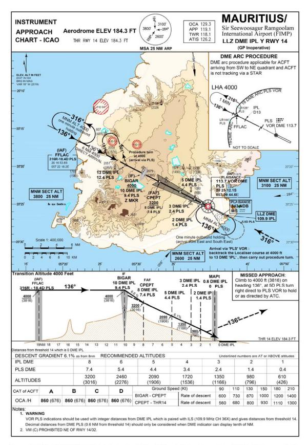
Changes: BIGAR is 4000, CPEPT is 3200, obstacle elevations 2058 and 1674, underlined numbers are AT or ABOVE altitudes concern Profile FFLAC is at 19nm from threshold in profile, ZMKR instead of FAN MKR at BIGAR
