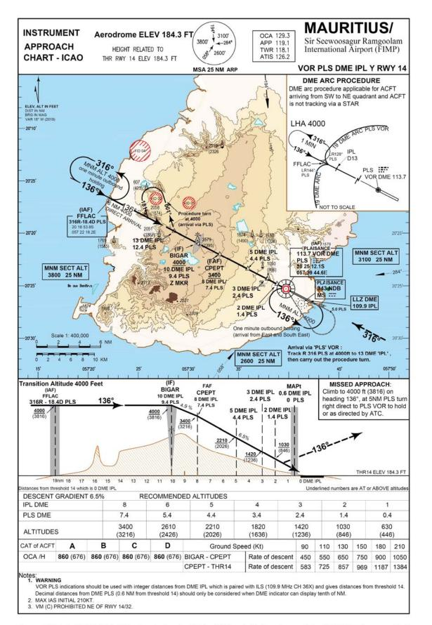
Changes: BIGAR is 4000, CPEPT is 3400, obstacle elevations 2058 and 1674, underlined numbers are AT or ABOVE altitudes concern Profile FFLAC is at 19nm from threshold in profile, inclusion of ZMKR at BIGAR instead of FAN MKR
