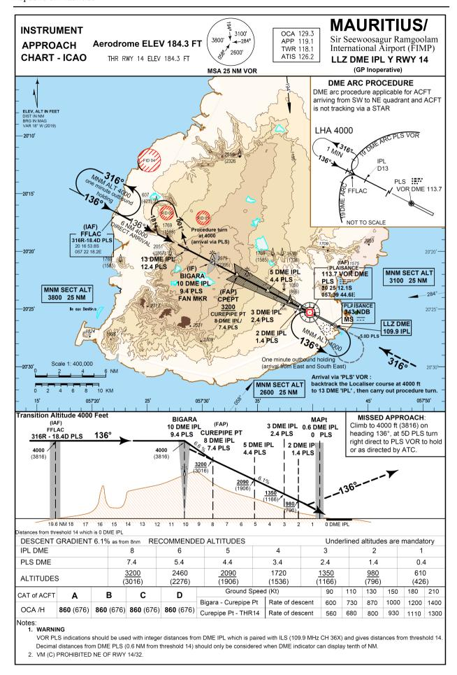
Changes: Changes: Removal of NDBs FF and MS, DME arcs, holding pattern and new missed approach procedure
