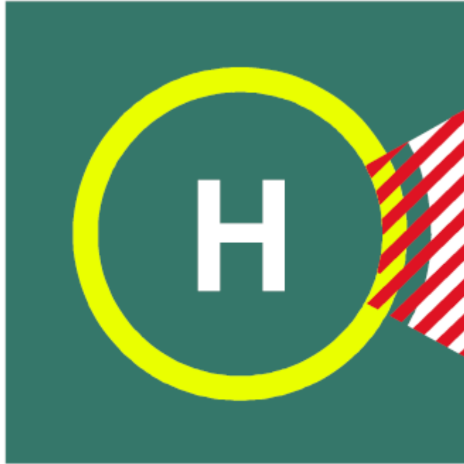
Figure 5-7. Helideck prohibited landing sector marking
