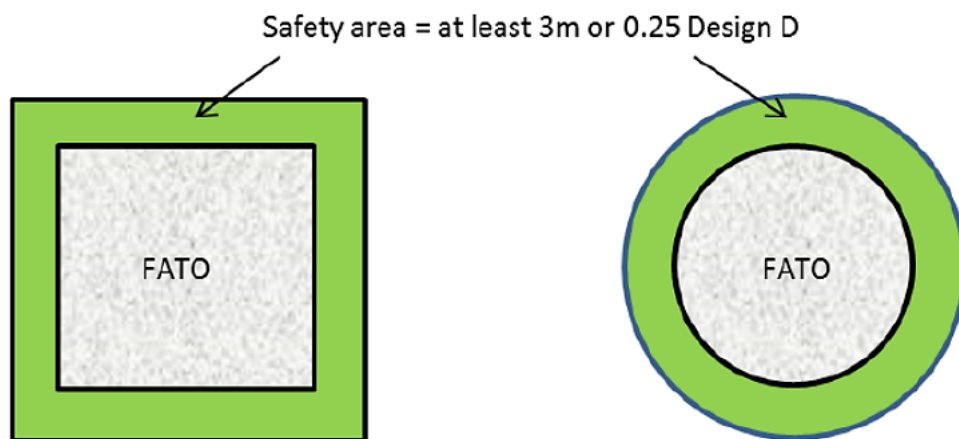
Figure 3-1. FATO and associated safety area
