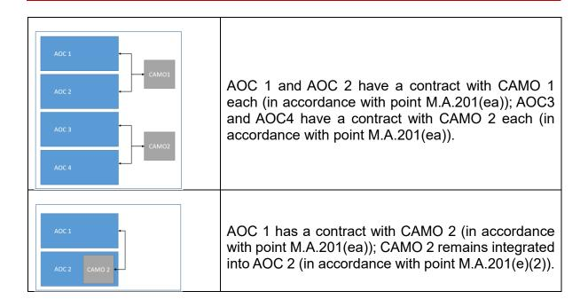
(c) The following schemes illustrate examples of configurations that are not compliant with point M.A.201(ea) (non exhaustive list):
