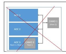
This configuration is not compliant with point M.A.201(ea) because CAMO 1 is not contracted by AOC 3 for all the aircraft it operates.
